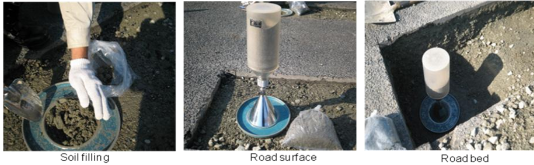
Photo 4: Field density test
